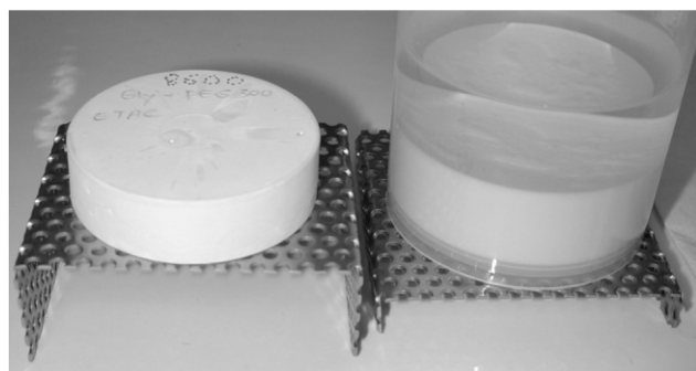
Fig. 1. Hyperporous polyurethane samples before (right) and after (left) direct supercritical CO 2 drying.
